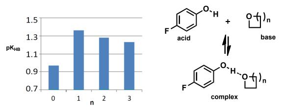
Figure: strength of association with 4-fluorophenol in cyclic ethers against ring-size
